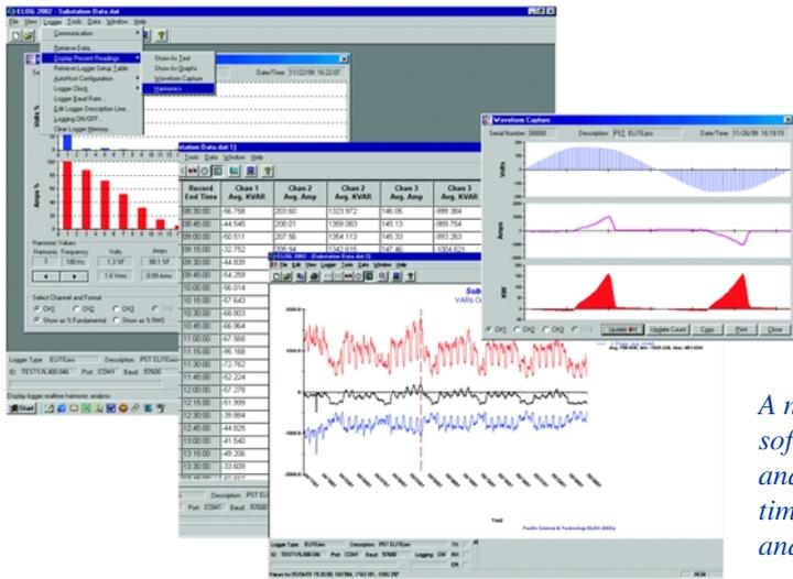
*A new generation of software allows intuitive analysis of usage over time, critical harmonics, and peak power demands.*
